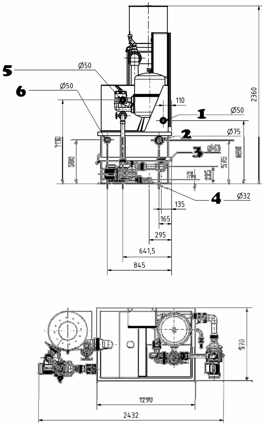
**Abb. 2: Systemfilter Skim Anschlüsse**
